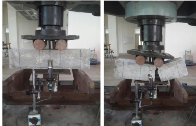
Figure 2. Two-point bending test.
